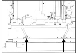
Figure 8 – IBT Condensation Drain Assembly Connections
